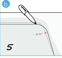
Mark template parts with the marker. If template line or part of the line need to be adjusted indicate the boundary of the adjustment, then use arrow mark to indicate inward or outward adjustment and amount of adjustment next to the arrow.
