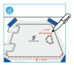
Amount need to have "+" sign for outward adjustment and "-" sing for inward adjustment. If adjustment tapers to the existing line indicate the point where the adjustment line touches original line with 0 amount and the adjustment amount on the other end of a new line.
